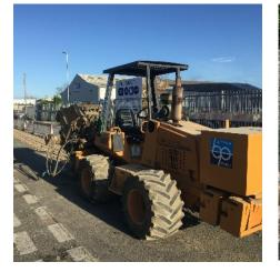
250 to 500 metres in length from each jointing bay. A Grundo Winch, Capstan Winch and Compressor were used to assist in the installation of the Electric Cable and the installation of the draw ropes. Competent, trained operators and operatives on site with constant radio communication and monitoring during each cable pull ensured continuity and successful installation.
